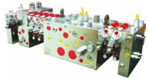
ABOVE: **Hybrid CV2000 – a highly customised valve assembly that has boosted machine performance while reducing the size of its hydraulic system**
