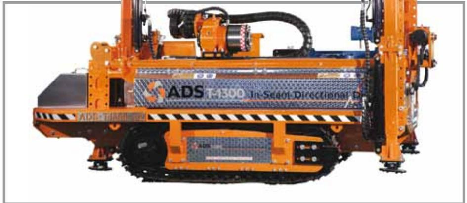
ABOVE AND BELOW LEFT: **Track-mounted horizontal drill for use in explosive atmospheres**
